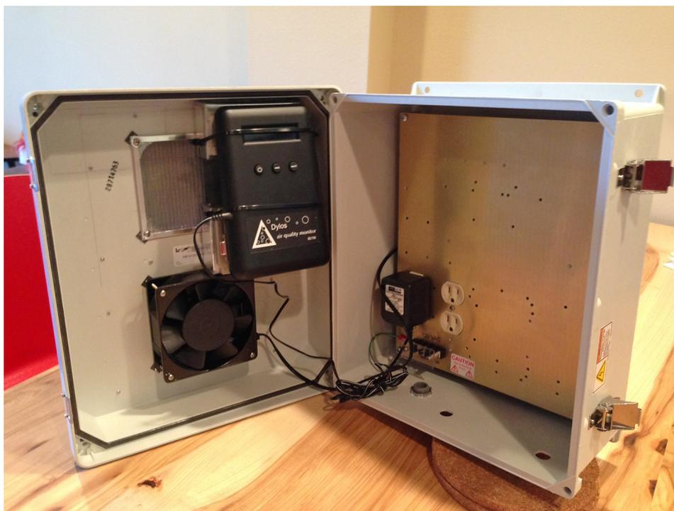
**Figure 2.** Air monitor system including modified Dylos particle sensor with four size bins ( $>0.5 \mu\text{m}$ ,  $>1.0 \mu\text{m}$ ,  $>2.5 \mu\text{m}$  and  $>10 \mu\text{m}$ ), temperature and relative humidity sensors, and a microcontroller.
