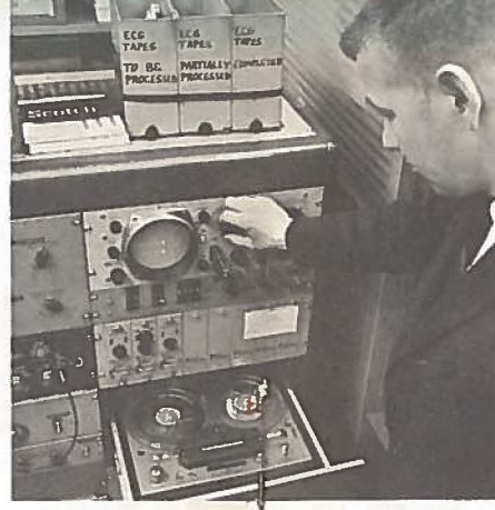
AT COMPUTER CENTER automatic receiving device accepts ECG signal and turns on analogue-to-digital converter (above), which feeds 500 numerical values a second into the digital computer. Results are automatically printed out on electric typewriter (below) in less than four minutes. Wave amplitudes are indicated in millivolts and durations in seconds; borderline or abnormal values are shown by asterisks.
